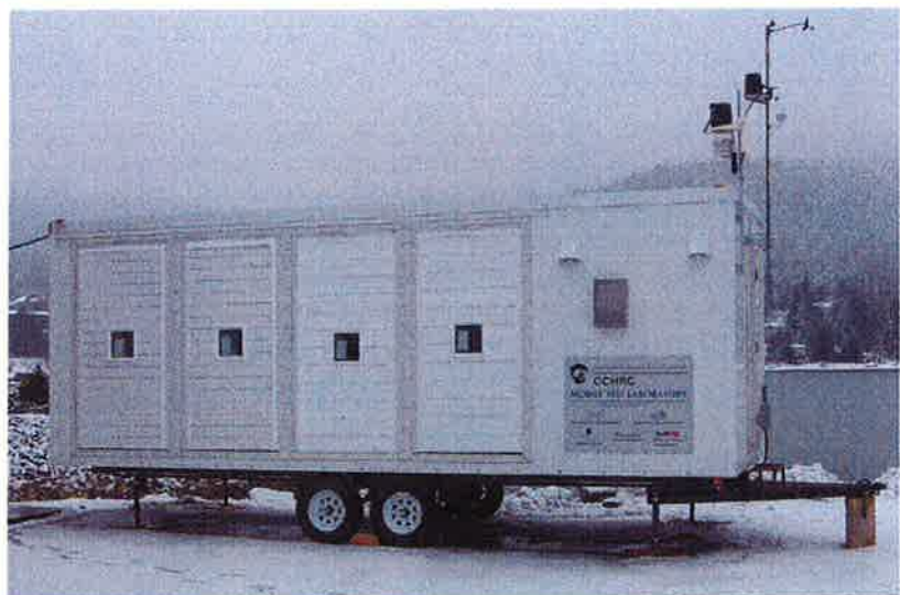
Mobile Test Lab with wall sections in Juneau
